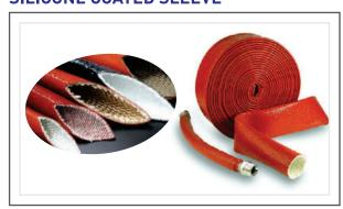
Knitted High bulk fiberglass sleeve can withstand repeated exposures to molten steel, molten aluminum and molten glass upto 3000° F (1650° C)
